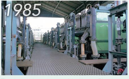
1985 The electrolysis equipment of the Nagoya Plant is changed to the ion exchange membrane method.
