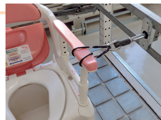
Armrest strength test
