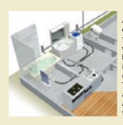
Aron Kasei has developed a centralized drainage system for single-family houses in which wastewater from the kitchen, washbasin, and bath is channeled through one pipe under the floor of the house. This reduces labor costs associated with installation as well as maintenance, and improves the system's efficiency.
