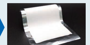
Composite membrane made of organic and inorganic electrolytes
