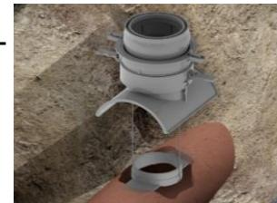
Convert a corroded aging pipe to a PVC pipe with a single joint
