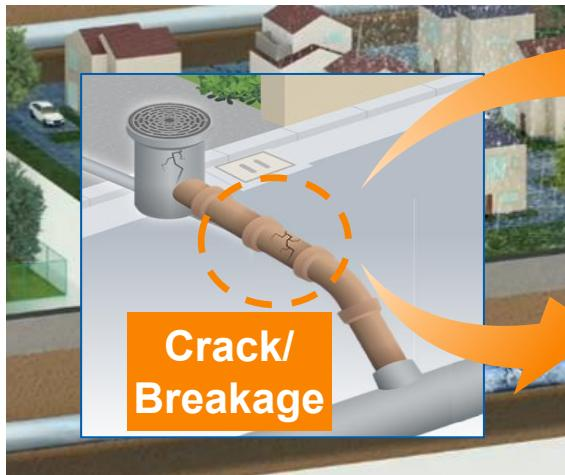
Joint at the water-leakage point for repair
