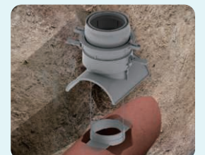
Joint at the water leakage point for repair
