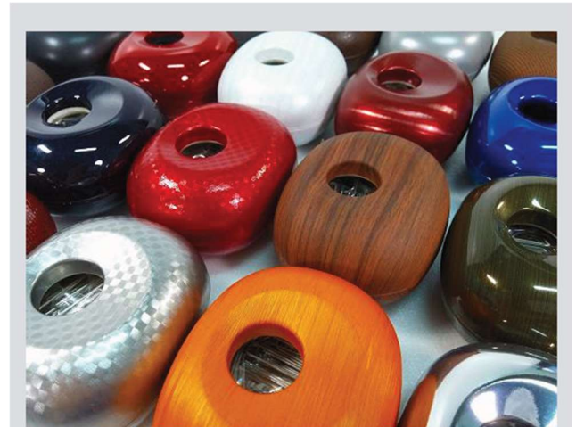
Figure 1: Example of film decoration by vacuum pressure forming 6)
