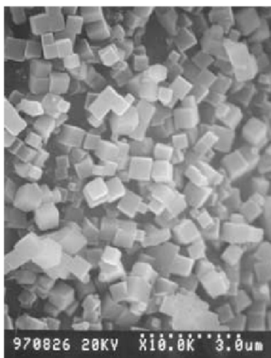
Figure 2: Scanning electron microscope photograph of NOVARON AG300
